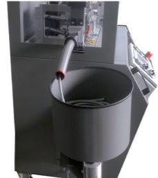
Fig. 3 Coiler pin with adjustable drive motor
